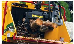
**CHIPPING PRODUCTIVITY.** The SmartFeed system monitors engine rpm and automatically stops and reverses the feed rollers to enhance production. This system also senses feed roller iams and manipulates the material automatically to reduce the need for manual feed control bar use.
