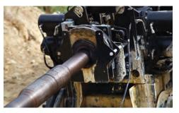
**VISE.** The sliding vise moves 35.4" (89.9 cm) to help operators position the vise for maximum efficiency when reaming or pulling product.
