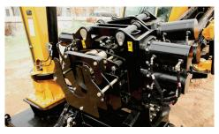
**OPEN-TOP VISE DESIGN.** Features an open-top vise design for the purpose of removing and adding tooling.
