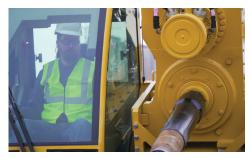
**DUAL-PIVOT RACK.** Allows for rack entry angles from 10 degrees to 24 degrees to help maximize the versatility of the rig for various product pipes and jobsite terrains.
