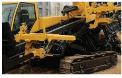
**OPTIONAL ROD LOADER.** A single-row, sliding-arm rod loader allows for the staging of five rods, helping increase boring efficiency by minimizing rod-loading time.
