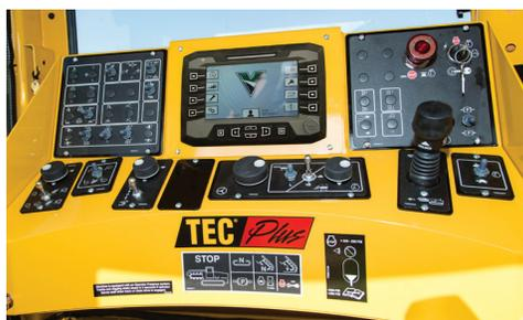
**SMARTTEC ELECTRONIC CONTROL SYSTEM.** SmartTEC performance monitoring assists operators with adjustments to machine controls to help improve efficiency and tracks the operational performance of the machine on a consistent platform across all machine models.
