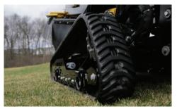
**NAVIGATE THROUGH NARROW SPACES.** When you need to navigate through narrow jobsites, you can retract the machine to only 35 in (89 cm) and then extend the tracks to 49 in (124.5 cm). The tracks are low disturbance, and they provide optimal traction and stability in tough ground conditions—leaving you with minimal job prep and clean up afterwards.
