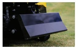
**OPTIONAL BACKFILL BLADE.** Minimize jobsite clean up with the optional backfill blade. It efficiently moves chips around the jobsite, reducing the need to manually relocate the chips. The blade has a rounded lower
