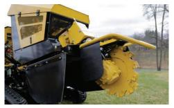
**MAXIMUM POWER.** To use all of its 48 hp (36 kW), there's the beltless direct-drive system. This delivers the maximum amount of power from the engine to the cutter wheel through a pair of gearboxes connected by a driveshaft. You can expect minimal maintenance cost, due to the beltless design of this system.
