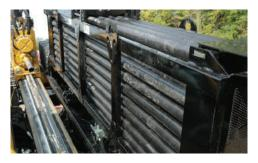
MORE FEET ONBOARD. Install more feet and save time with an impressive 500' (152.4 m) of drill rod on-board.
