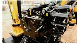
**OPEN-TOP VISE DESIGN.** Features an open-top vise design for the purpose of removing and adding tooling.
