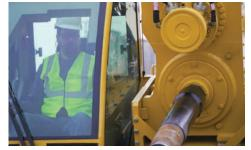
**DUAL-PIVOT RACK.** Allows for rack entry angles from 10 degrees to 24 degrees to help maximize the versatility of the rig for various product pipes and jobsite terrains.
