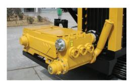
**OPTIONAL ONBOARD DRILLING FLUID** PUMP. 1136 L/min (300 gpm) for a self-contained drilling system. For larger projects, the onboard pump can be used in combination with a stand-alone pump if additional fluid flow is required.
