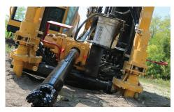
LESS RESTRICTIONS. A hollow inner rod design results in more air and drilling fluid flow to the drill head on pilot bores and the hole opener during pullback, providing contractors the ability to select from a more diverse range of tooling options, including air hammers and larger hole openers.
