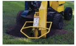
AUTOSWEEP® CONTROL SYSTEM. The optional AutoSweep control system monitors engine speed and automatically adjusts cutter wheel sweep rate, and is designed to reduce engine, drivetrain and structural stress.
