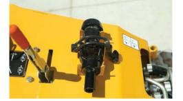
**PORTA BORING.** Easily transition from plowing to boring under driveways, sidewalks and other obstacles with an optional Porta Bore attachment.
