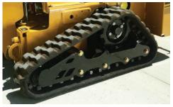
**DECREASE TURF DISTURBANCE.** Dual rubber tracks with a ground pressure of 3.7 psi (.3 bar) minimize disturbance and restoration to the jobsite while tackling tough ground conditions. This lightweight plow will also help save time with a 3.7 mph (6 km/h) transport speed.
