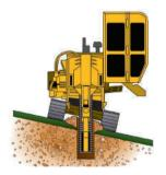
**OPTIONAL AUTO TILT TRACK.** An oscillating track frame allows the track to follow the ground's contour, providing a vertical trench on slopes up to 10.5 degrees.
