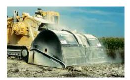
**TERRAIN LEVELER® SURFACE EXCAVATION** MACHINE ATTACHMENT. The T955III has a chain drive Terrain Leveler option for large rock excavation applications including surface mining, overburden removal, site preparation and road demolition.
