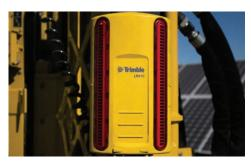
MAINTAIN ACCURACY. An optional laser receiver and an optional compatible third-party GPS system can provide visual input to the operator and input to the machine control system to help improve productivity and alignment of the machine to the specified pile location.
