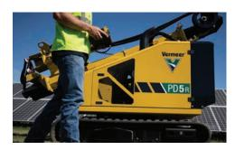
**COMPACT DESIGN.** A small machine with transport dimensions of 85 in (215.9 cm) wide, 8.2 ft (2.5 m) tall and a 15 ft (4.6 m) mast is ideal for jobsites with less space, or for multiple smaller iobs that require continual transportation of the machine. Quickly move around the jobsite and continue efficiency of installations, helping reduce time spent on setup, teardown and transportation.
