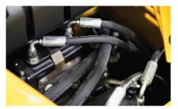
**MAXIMUM POWER.** The hydraulic pumps are attached directly to the engine giving the machine a greater power advantage over models directing power from the engine through the belt to the pump.
