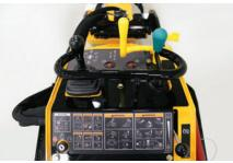
**STEADY TURNS.** A single, pilot-operated ground drive joystick offers a smooth range of motion without balancing engagement of two separate controls.
