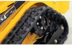
**LOWER YOUR COST OF OPERATION.** The undercarriage features a high-mounted track sprocket. The higher mounting reduces premature wear and tear in rocky soil conditions, while the cast sprocket is heat-treated for longer life.
