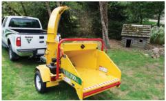
**THE LARGE INFEED OPENING** 6 in x 8 in (15.2 cm x 20.3 cm) makes feeding irregular material easier and decreases the amount of saw cuts needed prior to feeding the chipper.
