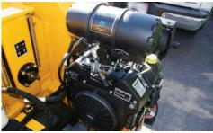
**25 HP (18.6 KW) EFI ENGINE** performs well during cold-weather starts, reduces occurrence of engine flooding and provides improved fuel economy over comparable carbureted gas engines.
