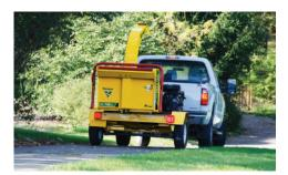
**THE WIDE AXLE** offers an ample footprint at the axle for side-to-side stability; additionally enhances transportability and visibility while backing up.
