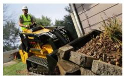
**OPTIMAL POWER.** Equipped with a 40 hp (29.8 kW) turbocharged Kohler KDI diesel engine. This engine eliminates the need for a diesel particulate filter (DPF), reducing cost and complexity of the engine.
