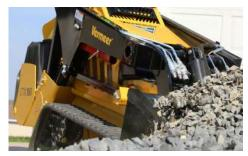
UNIVERSAL ATTACHMENT PLATE. The universal attachment plate provides maximized productivity by giving the operator the ability to change attachments on challenging jobs.
